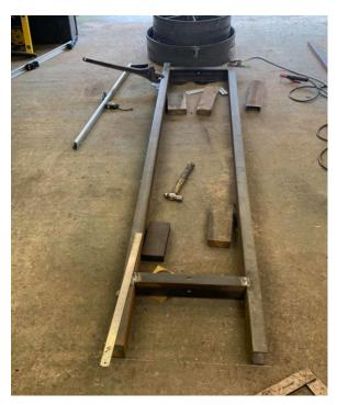
We decided upon a ladder chassis made out of 4" channel, 1/4" thick. The ladder chassis is 8' long and 20" wide, the beam axles are 3.5" box with 1 5/8" stub axles. We were going to need some substantial wheels to take the weight and I found a blacksmith in Ledbury called Alex Wilkins who makes steel wheels to order.
