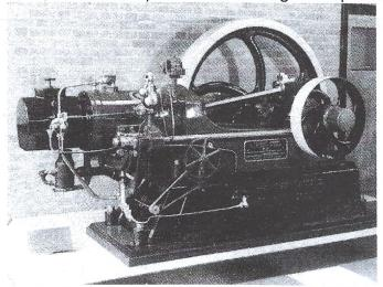
by the Explosion of Mixtures of Combustible Vapour or Gas and Air". This patent describes the World's first compression-ignition engine (*photo 1*).
