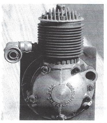
were never intended to carry lubricant in their crankcase, but must have survived on splash from cambox or gearcase, there being a ring of four slots to facilitate this in the inner crankcase wall. This inner wall supports a big (2" across), thin shell bronze bush and the other mainshaft is supported by a ball race in a blind housing. The crank itself is boringly normal except that the conn rod is cast bronze.
