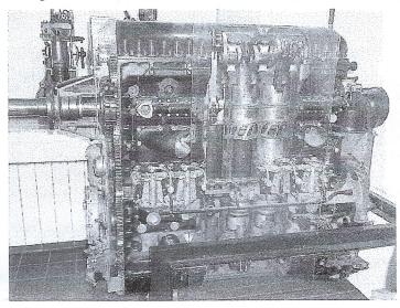
One of the main problems with high speed Diesels is to control and dissipate the heat entering the exhaust piston, and the liner round the combustion chamber and exhaust ports. The top of the piston in the Jumo was protected by a special heat-resisting plate, whilst a special type of " fire ring," without a split, is fitted beneath this plate and above the ordinary piston rings to protect the latter.
