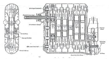
The engines worked on the opposedpiston two-stroke principle, but instead of the upper pistons being connected to the low crankshaft by long rods, as in another Junkers opposed piston engine, the Jumo aero engines had two crankshafts, one below the lower pistons and the other above the upper pistons. This arrangement reduced the inertia forces & thus permitted high speeds of operation and outputs, with corresponding higher specific reduction of weight.
