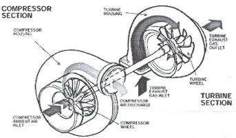
Briefly, the exhaust charge of expanding hot gas is put to driving a small turbine which is directly coupled to a compressor. This increases the pressure of the inlet charge to above atmospheric pressure.
