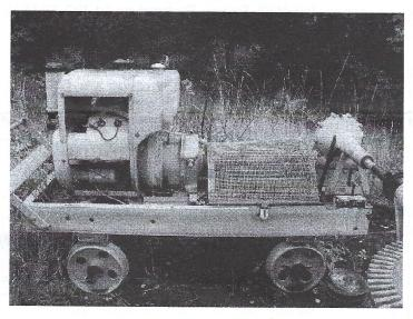
The vee four engine was introduced into the range in 1934 & in various models was in production until 1970. During this time, although the engine retained its basic configuration, the bore & stroke changed from 2 5/8" x 3 1/4" & ended at 3 1/2" x 4". The power output rose dramatically from 16 hp at 2,600 rpm to 60 hp at 3,600 rpm
